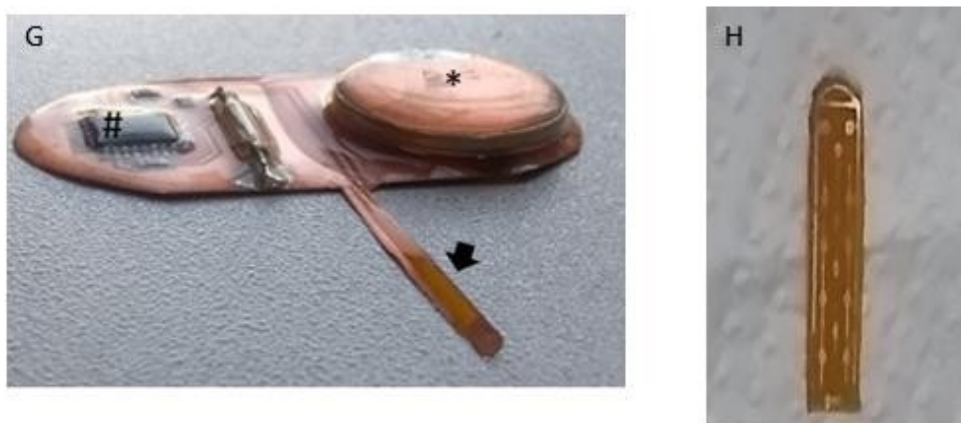
Figure 6. (A,B) bench test. Note the power supply adjusted to 5 V supplying the stimulation device; (C,D): oscilloscopic recording of the output current from the device (110 mV and 30.7 Hz). Figures (E,F) display the first version of the stimulator with its basic components, while Figure (G) depicts the final version of the device, # (Main microchip stimulation); * (Power supply); arrow (implantable electrode); (H) epidural implant electrode. The implantable pulse generator was designed and manufactured in our laboratory. It was conceived as a single piece, covered with dimethylpolysiloxane to avoid a battery leak. The lithium battery Sony CR2032, 220 mAh and 3 V, had enough charge to deliver a quadratic pulse of 30 Hz, 500 \mu s for 40 min a day over 60 days; the whole system required 1 mA/h. By the time of each animal's sacrifice, the device was explanted and battery tension stability was assessed by millimeter (always higher than 2.9 V).
